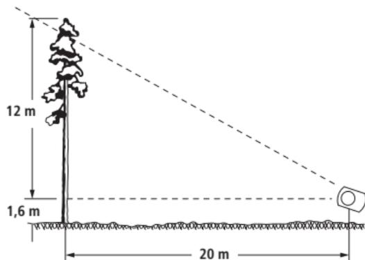
exactly correct result you have to proceed as stated below. On level ground, the tree top readings is usually sufficient: one only has to add the height of the observer's eye level (1,60 m in this case), which is already known.
